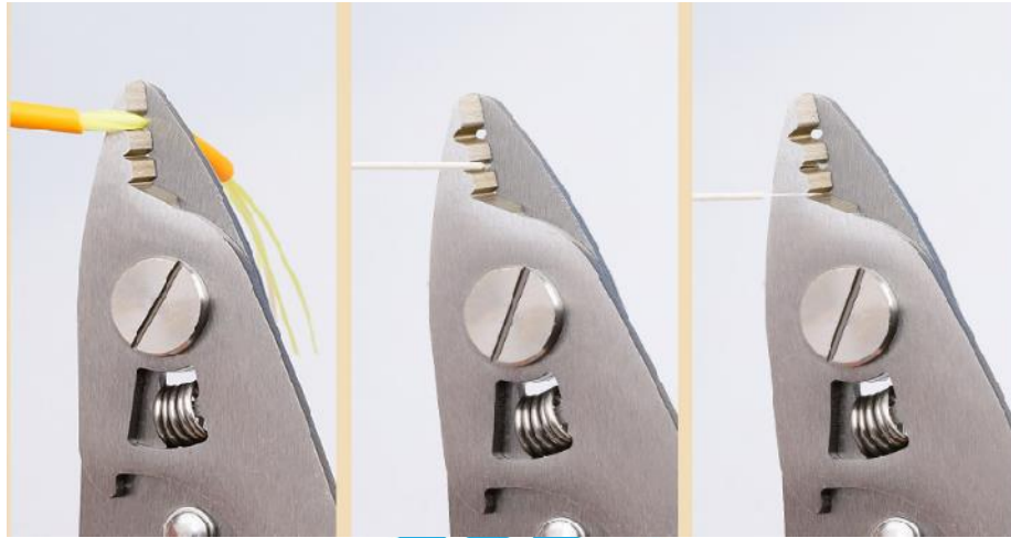
Figure 3.7 Preparation of patch cords
