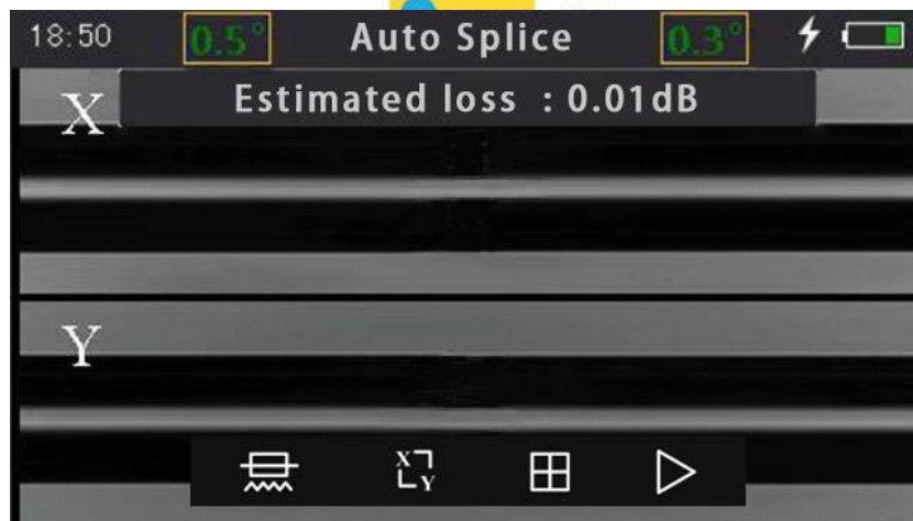
Figure 3.11 Completion of fusion splice
